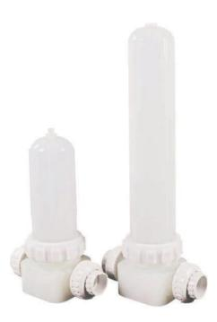
Micropore PP Filter Housing 226 type is made from pure polypropylene material, light weight and simple configuration design makes the installation and operation easier. The housing is designed to fit 10'' and 20'' 226 single open end cartridge. The material used is safe and low precipitation. It can be used in the filtration of water and general chemicals in kinds of industry.
